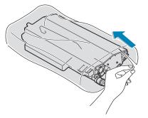
7 Remove the paper covering on the transfer belt by removing the tape.
